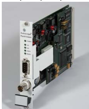
Figure 4: Single-camera RackVision processor
