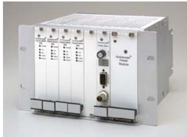
Figure 7: The Autoscope RackVision System RVS-4 configured for four-camera processing with the serial version of the Video Mux module and with optional Detector Rack Card
