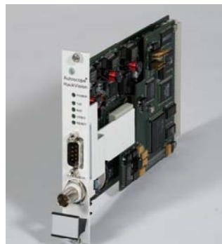
Figure 1: Euro Card version of the Autoscope RackVision single-camera Machine Vision Processor
