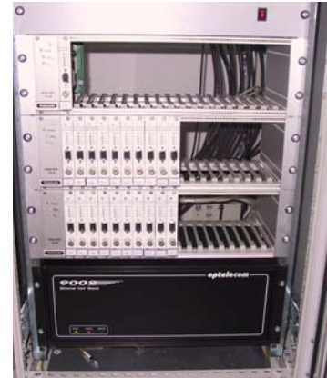
Figure 3: Autoscope RackVision Euro cards operating in Croatia
